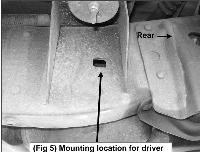
(Fig 5) Mounting location for driver side rear Mounting Bracket
